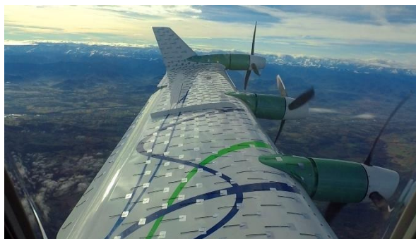
Wing view with the ePropellers activated
