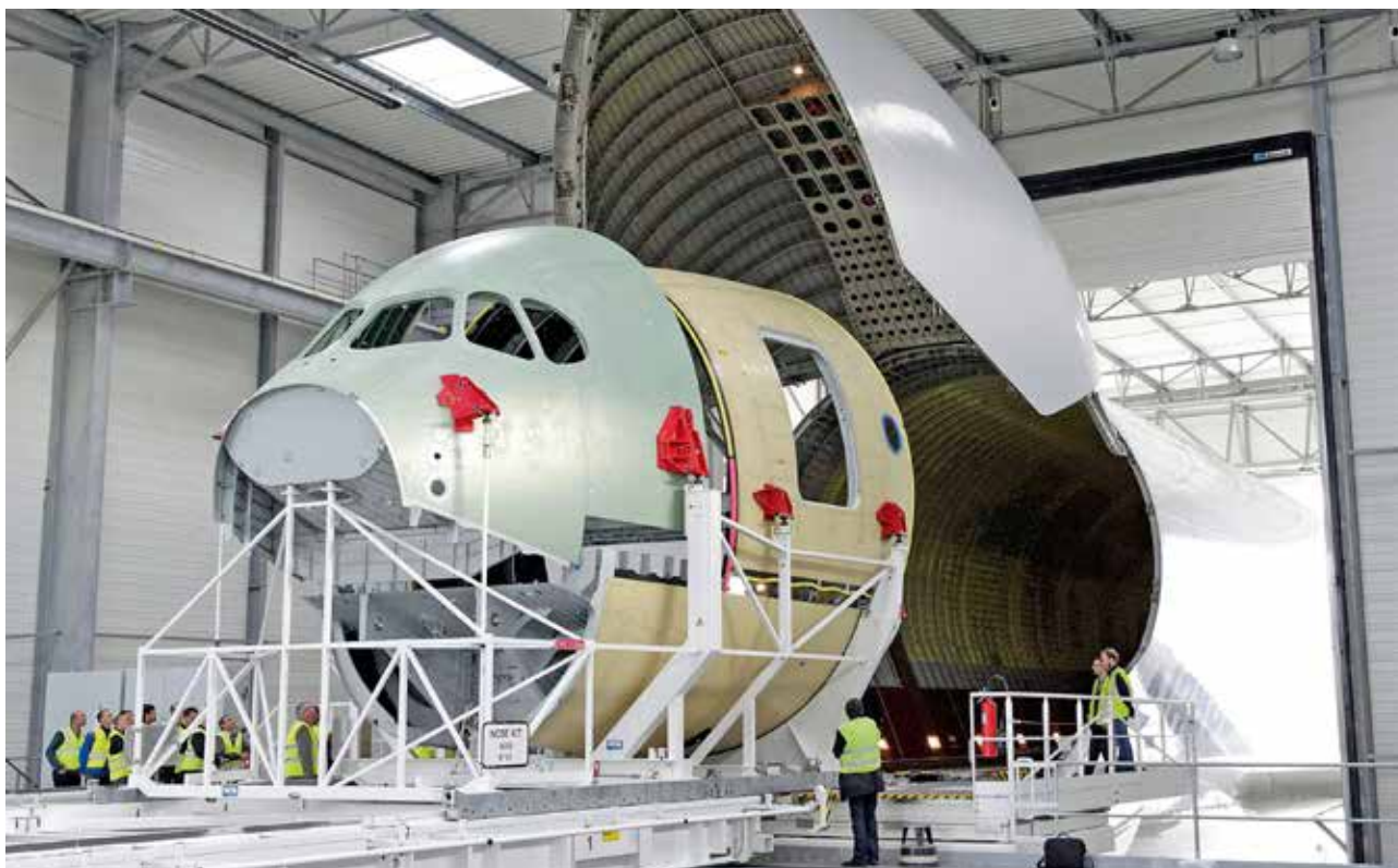
First A350 XWB nose section unloaded from a Beluga aircraft
